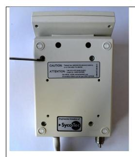
Unscrew 6x half-roundhead screws (pos.19) At the control unit with screwdriver Torx T8 (pos.20)
