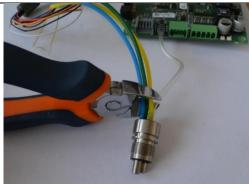
Cut off the media hoses with side cutter (pos.21)
