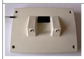
Loosen 4x half-round screws (pos.18) on display with screwdriver Torx T8 (pos.20)
