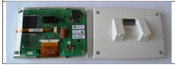
Display with removed cover at the back
